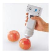
For even more user flexibility the measuring head, equipped with Display, function keys and power supply, can now be used as "stand alone" or directly interfaced to the PC to run with the optional QC software SpectraMagic NX.
