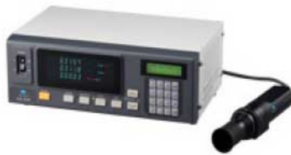
CA-310 (Using CA-P32 probe) Accuracy guaranteed range for luminance: 0.005 to 1,000 \text{cd/m}^2
