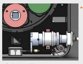
The ProMetric I-SC employs a mirror mounted inside the imaging colorimeter on the color filter wheel to redirect light through a fiber-optic cable to the spectrometer.
