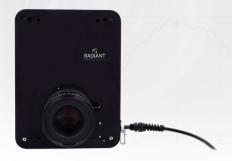
ProMetric I-SC imaging colorimeters, and the electronically-controlled lenses supplied with them, are factory-calibrated over all possible distances and two specific aperture settings. Because the lenses are electronically controllable for focus (working distance) and aperture, the colorimeter will automatically apply the appropriate flat-field correction.
